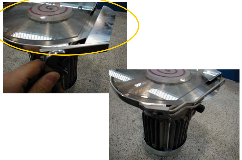
4) Replace the blade guard with the new guard supplied
