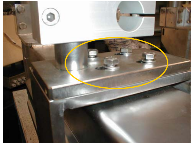
2) Fit back the projector/motor supporting bracket
