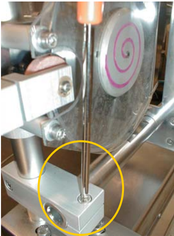
7) Remove bracket+photodetector support
