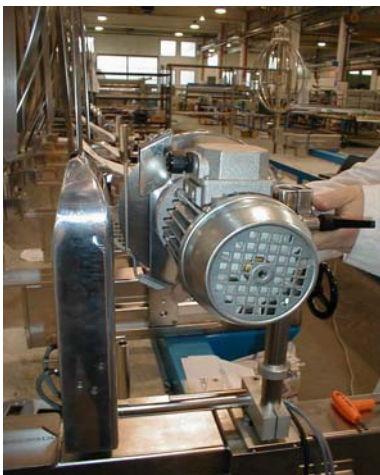
5) Fit back the engine assembly
