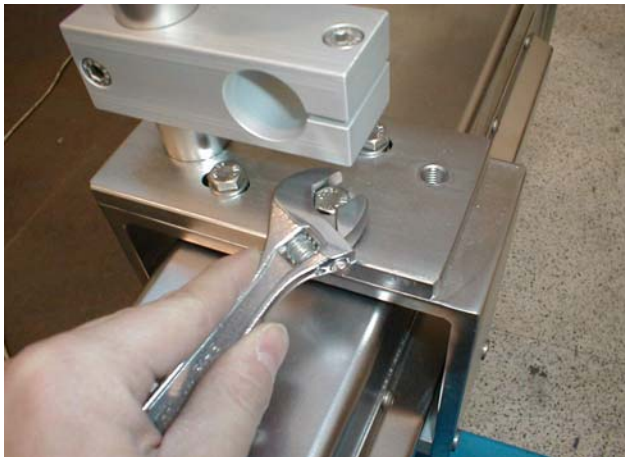
9) Remove bracket supporting motor/projector
