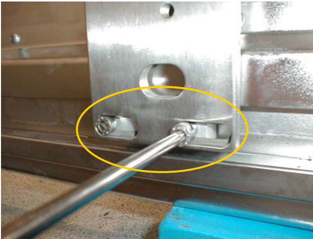
1) Install the U bracket towards the handwheel
