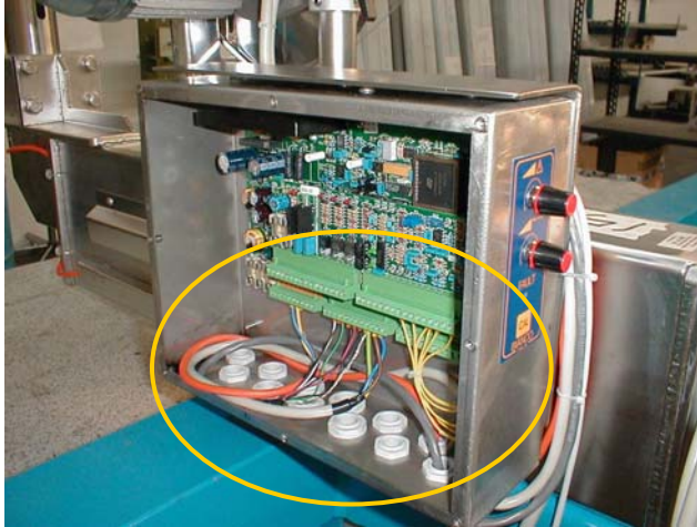
1) Disconnect the cables from the box fitted to the basket 2) Disconnect the limit switch and remove it
