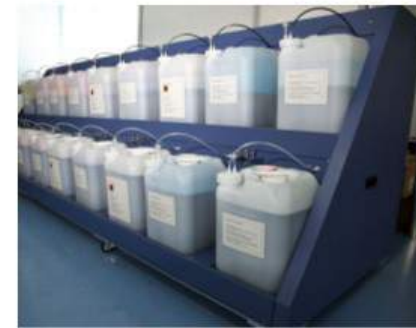
Bulk-feed system (with inline degassing)
