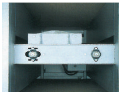
Prior to the last treatment chamber, the fabric passes through a steam and vibration section, which helps to enhance the fabric volume and soft fleecy handle.
